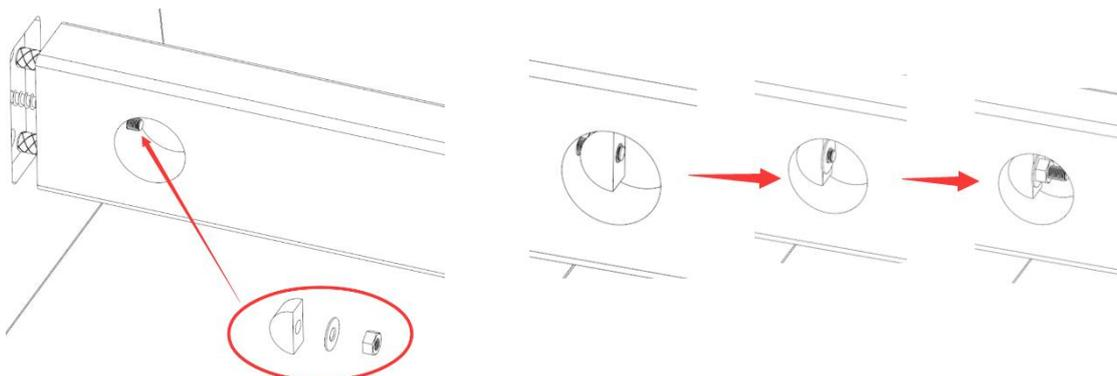
4) Same for the other side of the bases. Finally, use the black plastic cover the screw holes.
