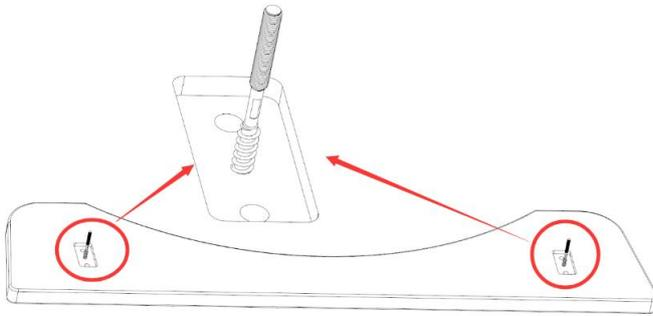
2) Connect the support beam with the base. The thread should go through the beam per the hole.
